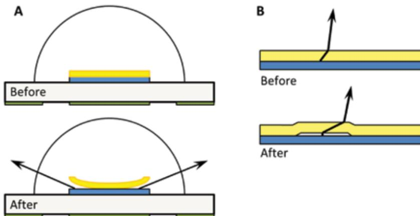
Curling (A) and delaminating (B, close up) are two potential causes of color shift with phosphor-coated LED packages. Curling generally causes a shift toward blue, whereas delaminating generally causes a shift toward yellow.
